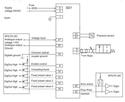
The example shows the controller as a pressure reducing control with throttle valves with 10-Bit analogue inputs (2-solenoid application). The preset value is issued by the PLC as a voltage signal. The actual value is fed back to the controller in the forme of a voltage signal of corresponding size.
