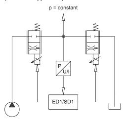
With this system, high dynamic and static requests can be performed. Any proportional valve with one active control edge can be used.
