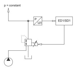
This system is actually only a electronically preset value re-lead. The problem is that the pressure already is mechanical controlled inside the valve. Because this mechanical control is very slow, the electronically control must be made slow artificially (cascade control: the exterior loop must be slower than the interior loop). With such a system, good static requests can be performed. However, dynamic requests can be badly performed.
