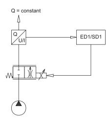
With this system, high dynamic and static requests can be performed. Any proportional valve with one active control edge can be used.
