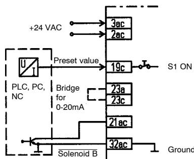
Connection of the preset value module with switch or PLC, PC, NC
