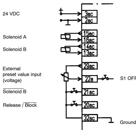
Supply voltage 24 VAC, preset value pre-setting with current. Solenoid B change with PLC, PC, NC
