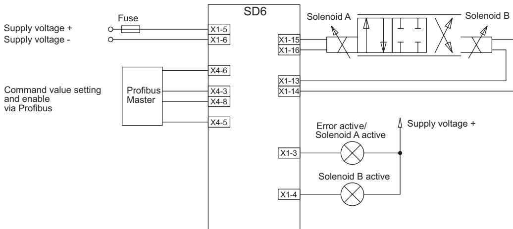
**Operating mode 4** (Command value inputs: Fixed, both voltage)
